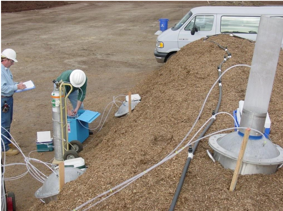
Figure 5. Photo of flux chamber set up used for compost pile VOC and NH 3 emission estimation (CIWMB, 2003).
